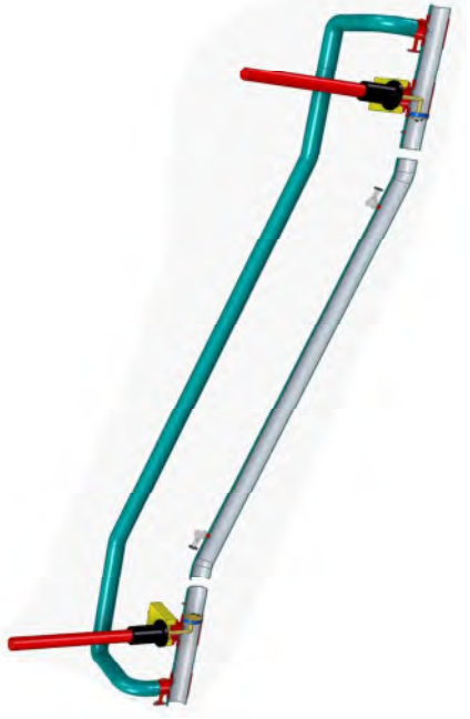
Fig. Cold-Cutting of Header Pipe.
