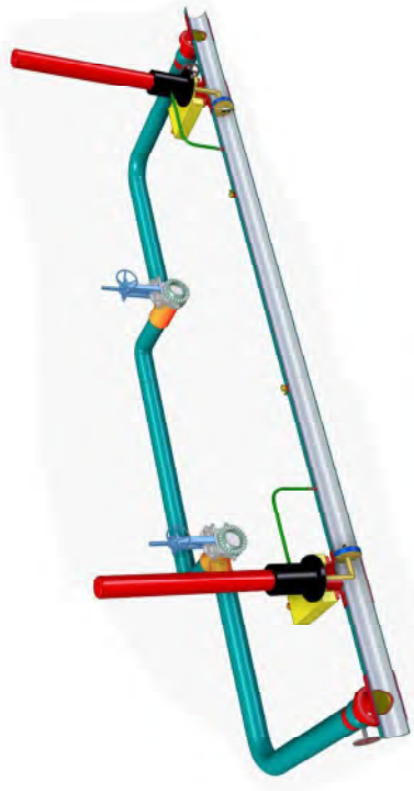
Fig. Insertion of Upstream Stopple Plug into Pipeline.
