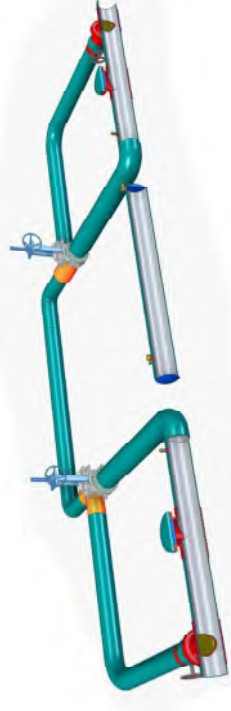
Fig. Permanent Line Blinding using Completion Plugs and Blind Flanges
