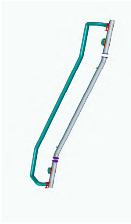
Fig. Permanent Line Blinding using Completion Plugs and Blind Flanges
