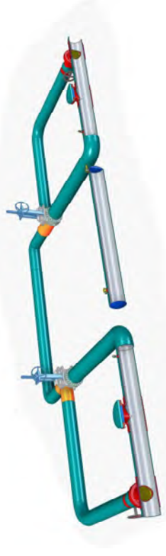
Fig. Re-Commissioning of Header line using 2" TOR Fitting
