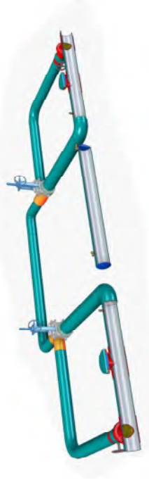
Fig. Stopple Plug Retraction
